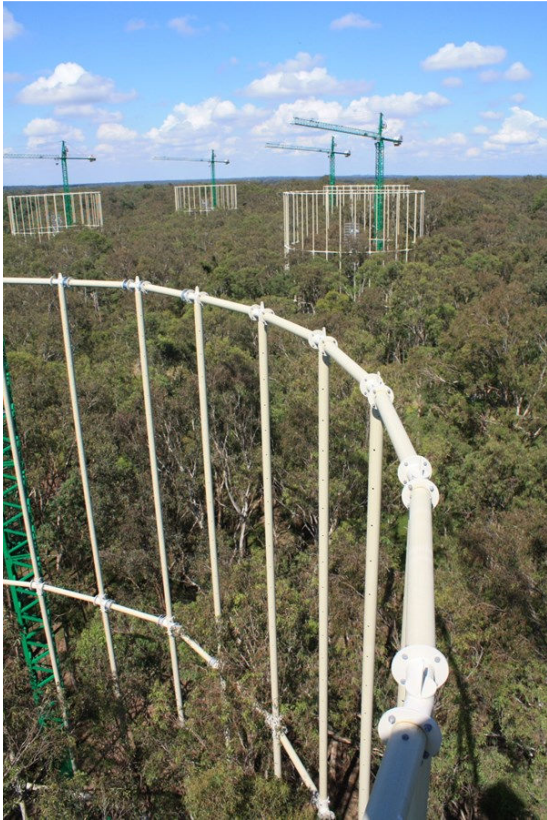
The Eucalyptus Free Air CO2 Enrichment experiment ( EUCFACE) located in the Cumberland forest
